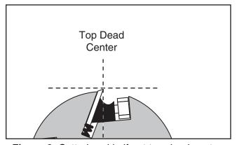
Figure 8. Cutterhead knife at top-dead-center.
